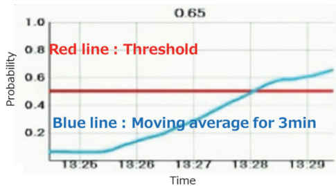
Fig. 6 An example of predictive detection of moving coil 2)
