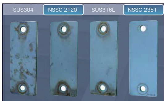
Fig. 17 Exposure test results of duplex stainless steels for 1 year in Southeast Asia ocean 62)
