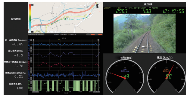
Fig. 7 Examples of measurements using video
