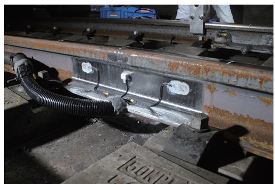
Fig. 4 Rail for contact force between wheel and rail measurement
