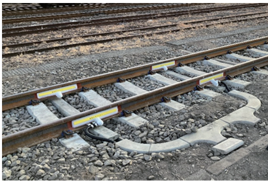
Fig. 5 Sensor for wheel load measuring device
