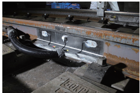
図4 地上輪重・横圧測定用センサー設置状況 Rail for contact force between wheel and rail measurement
