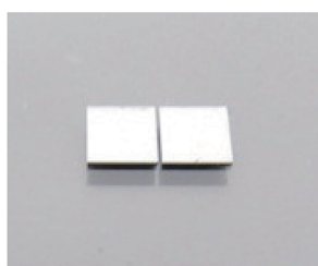
(a) Chip mounting image Mounted in parallel at 100 \mu m intervals
