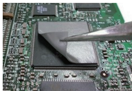
図10 放熱シートイメージ High thermal conductive silicone sheet with high thermal conductive pitch-based carbon fiber
