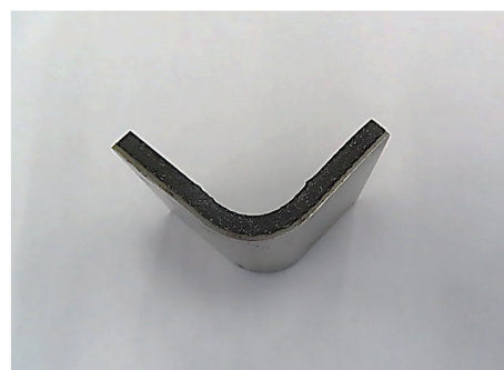
図2 一体成形加工後のCFRP複合鋼板の外観 Appearance of CFRP and steel composite after press forming
