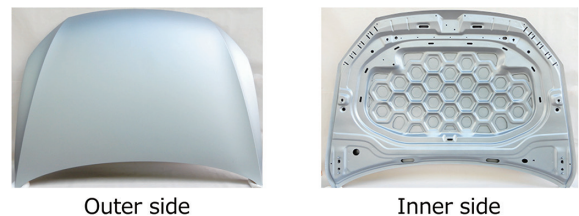
図 2 軽量フード試作品外観 Appearance of the prototype of lightweight-designed hood
