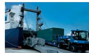
A roll trailer exiting via the rampway
