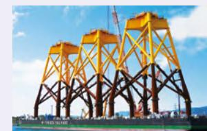
Jacket-type foundation to support offshore wind turbines
