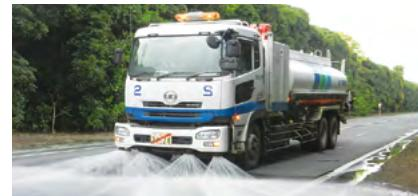
These trucks spray water on the road and empty lots or clean the road within works to restrict the secondary scattering of dust.
