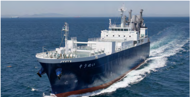
[High efficiency] • Adoption of roll trailers (load capacity: 60 tons) enables the transportation of heavy cargo. • A two-tier cargo structure has been introduced, equipped with a large elevator (210 tons per lift).
