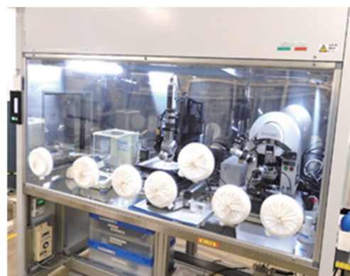
Fig. 3 Dry booth for LIB materials analysis (DP < -60^\circ\text{C} )
