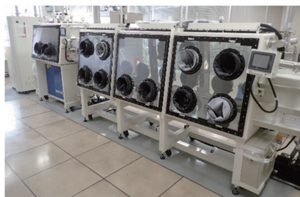
Fig. 2 Glove box for LIB prototyping (DP < -90^\circ\text{C} )
