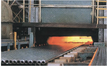
Heat treatment furnace
