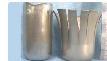
NSSC FW™2 SUS304 (Single cold rolling) Blank dia: φ80mm, Lubricant: JW#122 Punch dia (mm): 1st φ40→2nd φ35→3rd φ30→4th φ25
