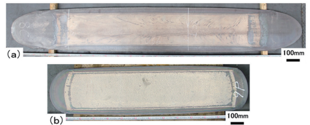
図6 大型梱包体を熱延したチタン厚板の外観 (a) 厚さ 15mm 13) , (b) 厚さ 40mm 12) Appearance of trial titanium plate made by hot rolling from large titanium package (a) 15 mm thick plate 13) , (b) 40 mm thick plate 12)
