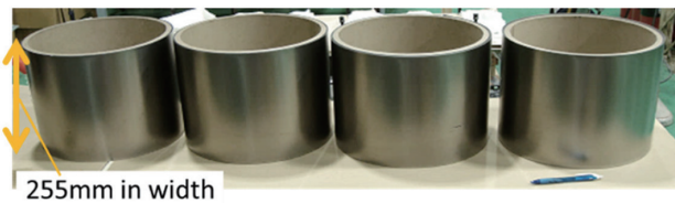
図7 試作したチタン薄板コイルの外観 Appearance of cold-rolled titanium coils made in the laboratory
