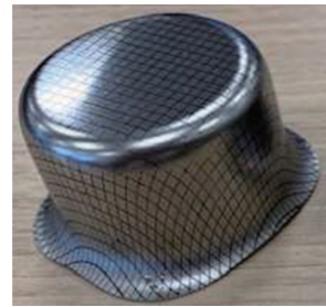
図6 Super-TIX ® 51AF 薄板深絞り後の外観(板厚 0.4mm, 絞り比 2) Photograph of Super-TIX ™ 51AF cold rolled sheet after cold deep drawing
